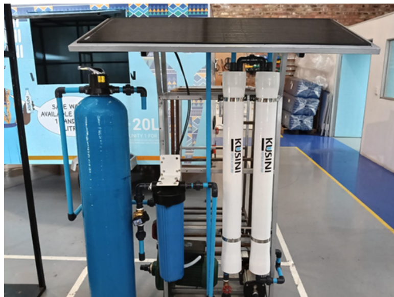
Figure A5.3: Kusini water filtration system combining solar, reverse osmosis and ultrafiltration technologies.
