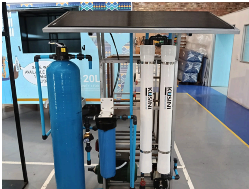
Figure 8: Kusini water filtration system combining solar, reverse osmosis and ultrafiltration technologies.
