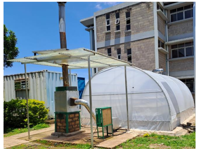
Figure 1: The hybrid solar dryer designed, fabricated, and installed by KIRDI
