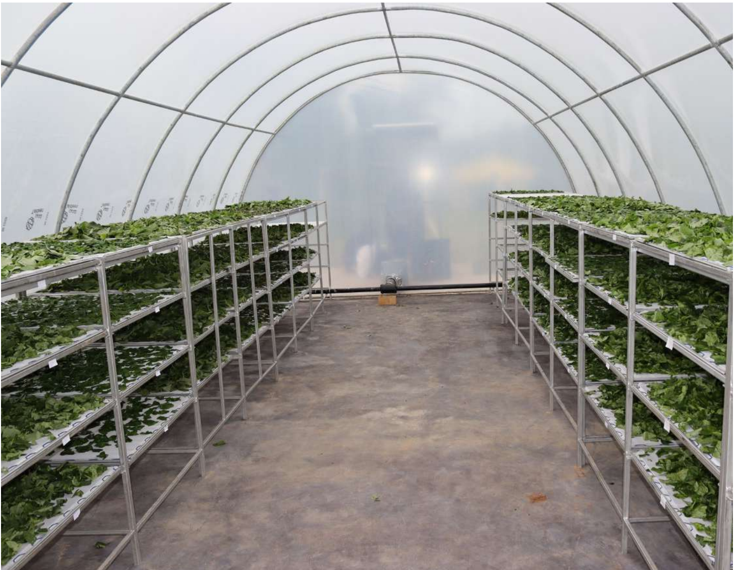
A prototype hybrid solar dryer that was installed in Kitui County. This is part of a project of scaling solar drying to reduce post-harvest losses in Kenya.
