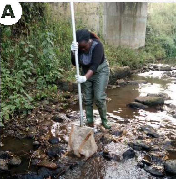
Plate 2: Demonstration of STEP 2 - Positioning the kicknet (A) and kicking the riverbed (B) for macroinvertebrate sample collection (Photos by Lorine Omondi (A) and Nzula Kitaka (B) )
