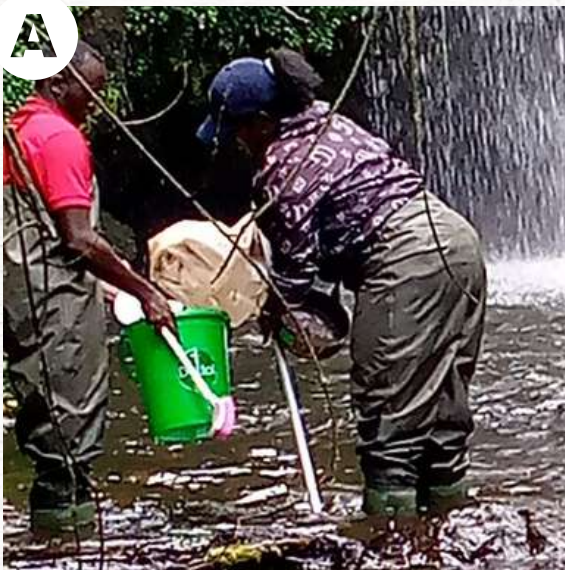
Plate 3: Demonstration of STEP 3 - Removing the sample from the kicknet (A) and washing of the net (B) (Photos by Nzula Kitaka)
